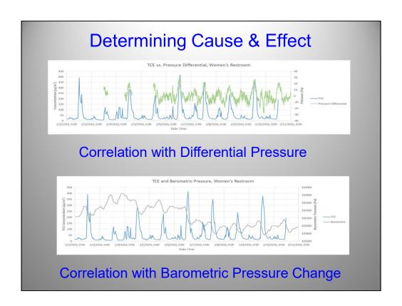
Comparison of the indoor TCE values to sub-foundation pressure shows a direct correlation between indoor air concentrations to positive pressure under the slab.
