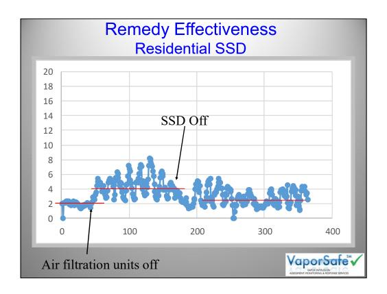
TCE indoor air concentrations in a home. The home was equipped with both a sub-slab depressurization system (SSD) and an indoor air filtration unit. The indoor air values were still at levels of concern. After a few days of monitoring, the air filtration units were turned off. Values increased and showed a sinusoidal pattern. After another 10 days, the SSD was turned off after 2 weeks (run #180) and the indoor air concentrations DECREASED!!
