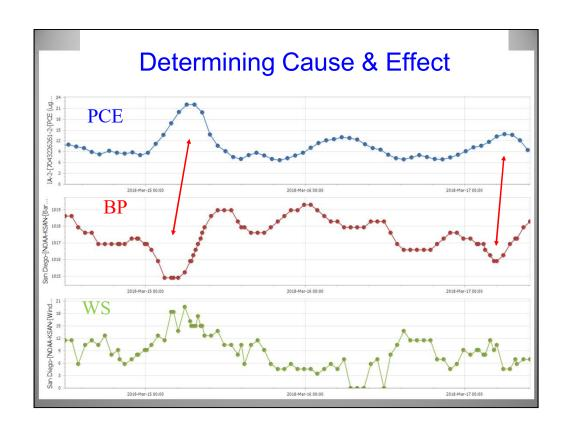
PCE indoor air concentrations in an office building which was formerly a dry cleaner. Definite correlations exist between the indoor air PCE values and dropping barometric pressure. The office building contained a janitor closet with a floor drain which was concluded to be the PCE entry pathway.
