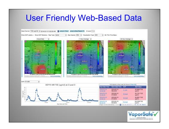
A picture of the user-friendly interface. Contour plots, plots of concentration versus time, stacked plots, and auto-alerts are all available from the dashboard. Plots can be easily exported into a jpeg file or into a ppt for rapid display to interested parties. Data can be easily downloaded in cvs or xls formats.
