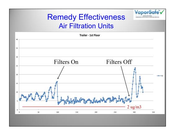
Indoor air concentrations of TCE in a double-wide trailer with a skirt underneath the trailer floor. Two indoor air filtration units were installed as a remedy to high TCE values (5 to 15 ug/m3). The filters decreased the indoor air TCE concentrations, but not below allowable levels. Another remedy had to be selected.
