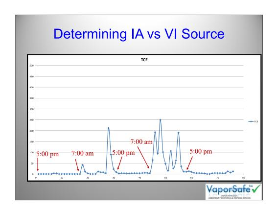
TCE indoor air concentrations in a furniture manufacturing facility. Concentrations were low at night, but then increased during the work day. If vapor intrusion was the source, values should have increased at night when the facility was closed up. The opposite was observed. It had to be coming from an inside source. What was the TCE source? On-site discrete sampling with the system found the hidden source.
