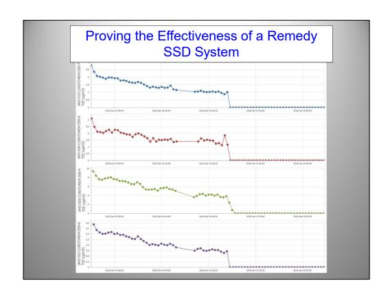
TCE indoor air concentrations at 4 locations in an operating facility. Note instant drop in indoor air TCE concentrations when the mitigation system was started-up and to levels that were far below allowable levels. The consistent low TCE values over the next 3 days was proof of the effectiveness of the system over the footprint of the building.
