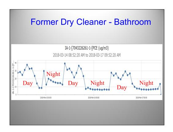
PCE indoor air concentrations in the same office building, but in the bathroom. High, variable levels during the day, but lower, stable values at night. What could be causing this pattern?
