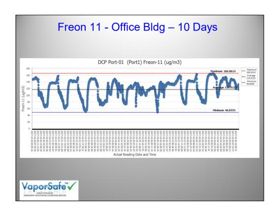
Freon-11 in indoor air over 10 days in the office building. The pattern was consistent from day to day and was a result of the HVAC system.
