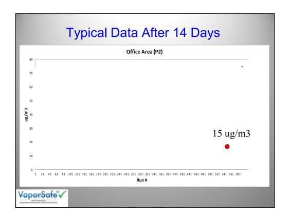
The dot in red shows the result if you had deployed a time-averaged sample for 14-days. The single value would have been biased high & indicated a problem. A false positive.
