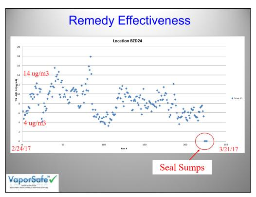
TCE concentrations in a basement at an industrial facility. Values ranged from 4 ug/m3 to 14 ug/m over the 1-month sampling period. But when two floor sumps were sealed up, values dropped to zero within a couple of hours. The monitoring data documented that this remedy would be effective and plans were made to seal the sumps permanently.
