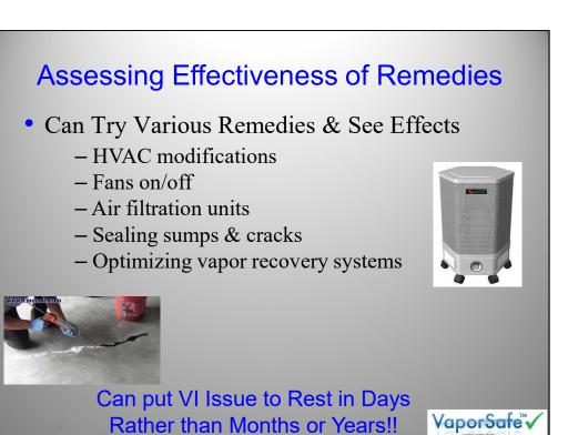
Monitoring data allow real-time evaluation of the effectiveness of a remedy. Adjustments to HVACs, vapor recovery systems, indoor air filtration units, exhaust fans can be made and the results seen in real-time.
