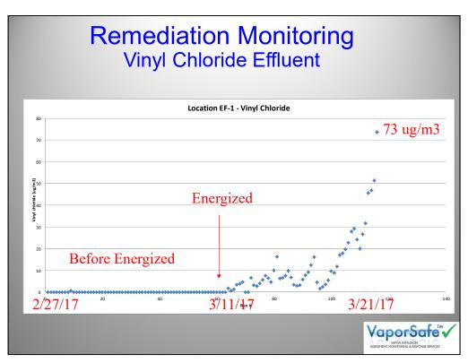
Vinyl Chloride in the effluent from a permanganate scrubber located immediately adjacent to a large thermal remediation project. The vinyl chloride concentrations started increasing almost immediately once the electrodes were energized. Vaporsafe data enabled rapid recognition of this situation and enabled the consultant to take immediate corrective action.
