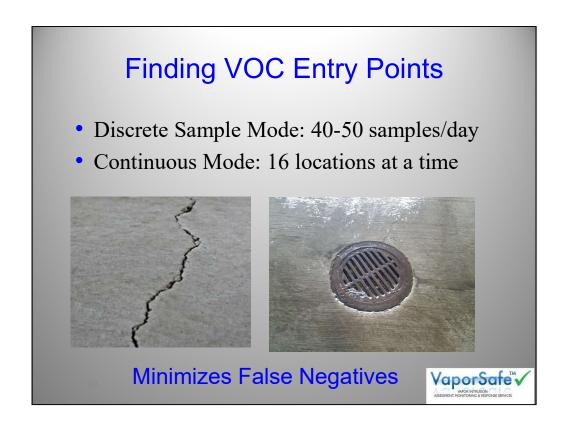
A huge benefit of the system is the ability to locate VOC entry points in a building. This can be done in either discrete sample mode or in automated monitoring mode.
